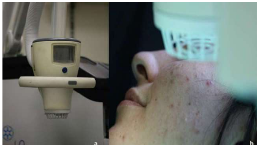
Fig. 1. Argon-CAP device used to irradiate affected skin areas of the face in each patient (a). The device consists of a torch operated at microwave excitation and production of an argon plasma (b).
